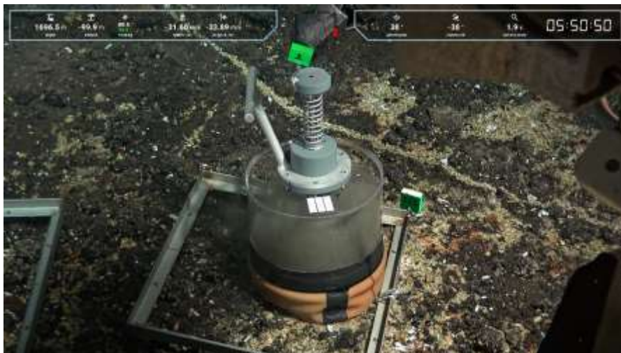
Figure 3. Deployment of the SPIDER particle spreader on a Bathymodiolus azoricus assemblage. Sulphide particles were spread over the fauna and the chamber was left for ~96 hours. Then, the fauna was recovered and conditioned for different analyses. Collaboration Ifremer/University of Açores/University of Algarve.
